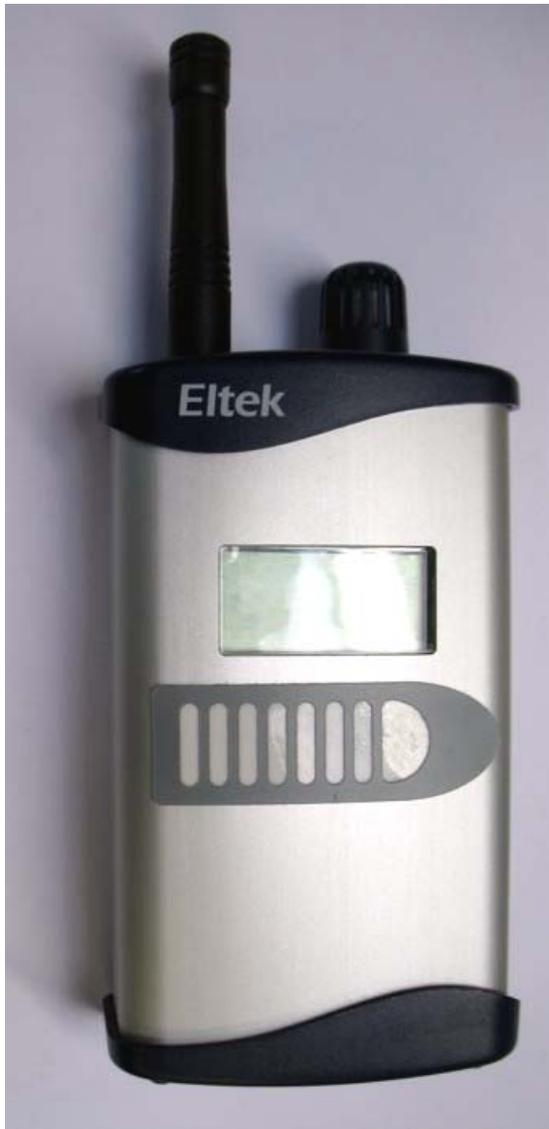
The GD47 transmitter is self contained air quality monitoring transmitter, with built in sensors for RH, temp and CO2 (0-2000ppm or 5000 ppm) for use with:-
